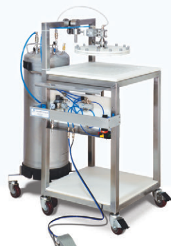
LIQUID INJECTOR FOR 3 LECHES CAKE. 150 cakes x hr 0.5 Oz up to 50 qt
